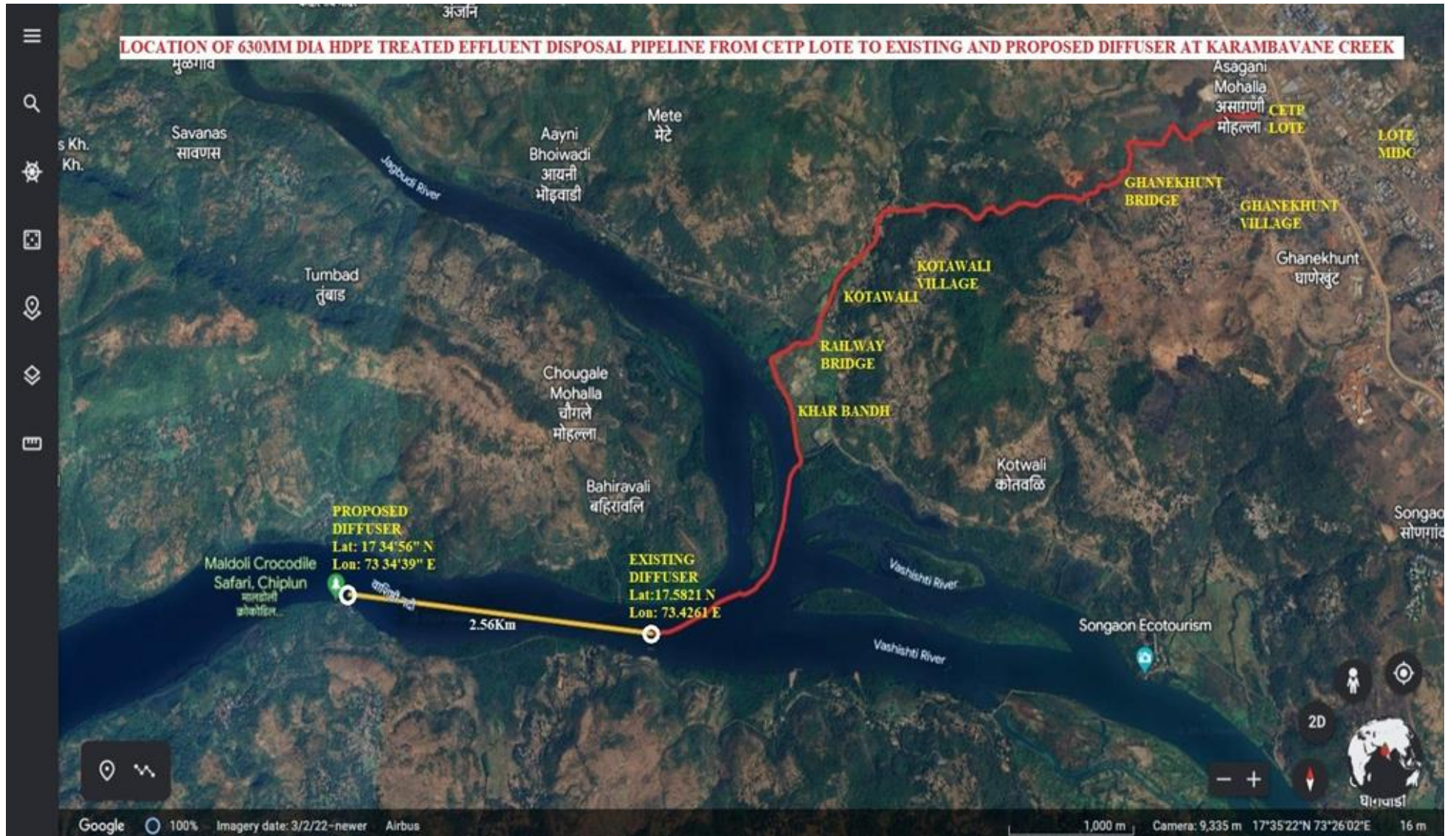
IMAGE-05 TREATED EFFLUENT DISPOSAL PIPELINE PATH
